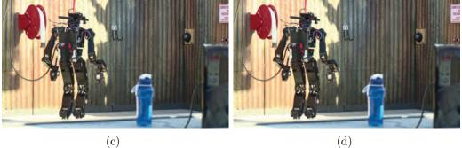
Figure 7.8: DRC-Hubo performing a hose installation task in DRC trial 2013.
