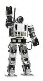
Figure A.2: Custom designed miniature humanoid robot for testing-and-evaluating, Mini-Hubo
