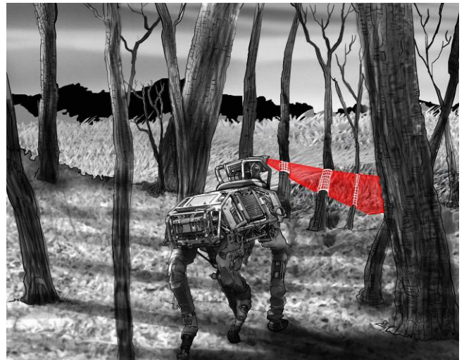
Figure 7. Concept for autonomous cross-country operation guided by computer vision and/or LIDAR, without human intervention. BigDog's rough-terrain control and reflexes will combine with terrain sensing to provide a high level of autonomy.
