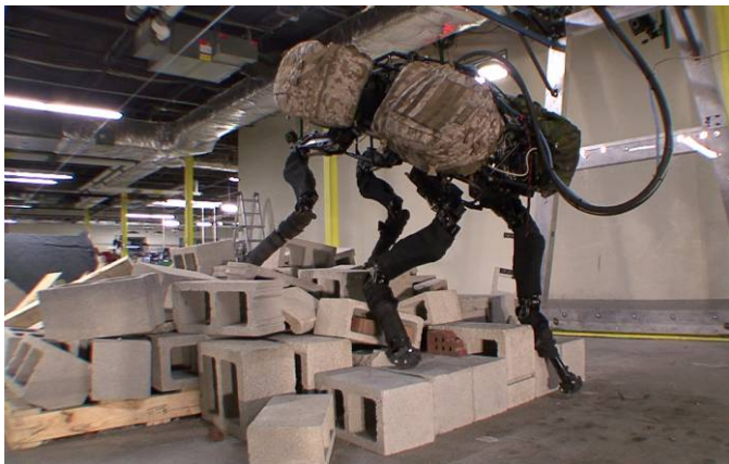
Figure 4. Top: BigDog climbing 35 degree slope with loose scree-like surface. The front legs were reversed for this experiment. Bottom: BigDog climbing a simulated rubble pile using a crawl gait in the laboratory. For this experiment, all terrain sensing is done with the legs, feeling its way along.
