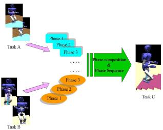
Fig.1.The overview of method for extended Task generation, such as stair climbing by Phase recomposition and Phase Sequence.
