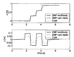
Figure 11: Modified ZMP of multibody model
