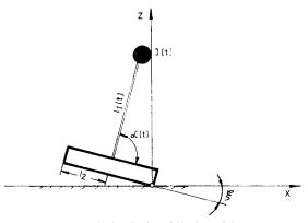
FIG. 15. Equivalent biped model.
