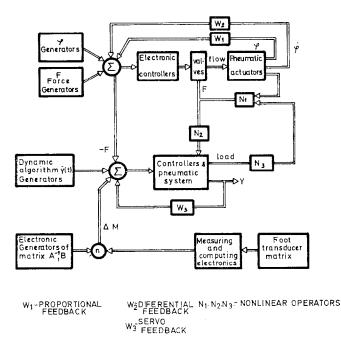
FIG. 18. Preliminary organization scheme of biped locomotion special purpose computer.
