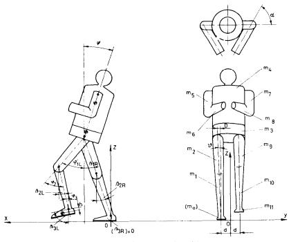
FIG. 3. Mechanical biped model.
