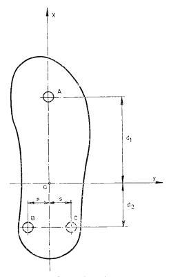
FIG. 9. Schematic illustration of vertical reaction components measurement.
