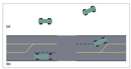
Figure 2. The importance of context for urban driving: (a) Without any context, the two vehicles appear to be on a collision course. (b) Given the context, we can safely assume that one of the vehicles is just making a lane change.
