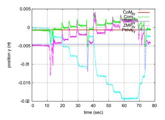
Fig. 6. CoM-ZMP movement with control and mass augmentation in loading objects
