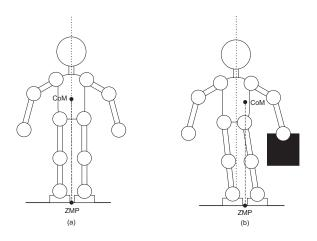
Fig. 1. CoM and ZMP relation (a) without and (b) with an object
