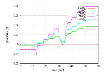
Fig. 5. CoM-ZMP movement with control but no mass augmentation in loading objects
