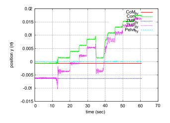
Fig. 4. CoM-ZMP movement with no control in loading objects
