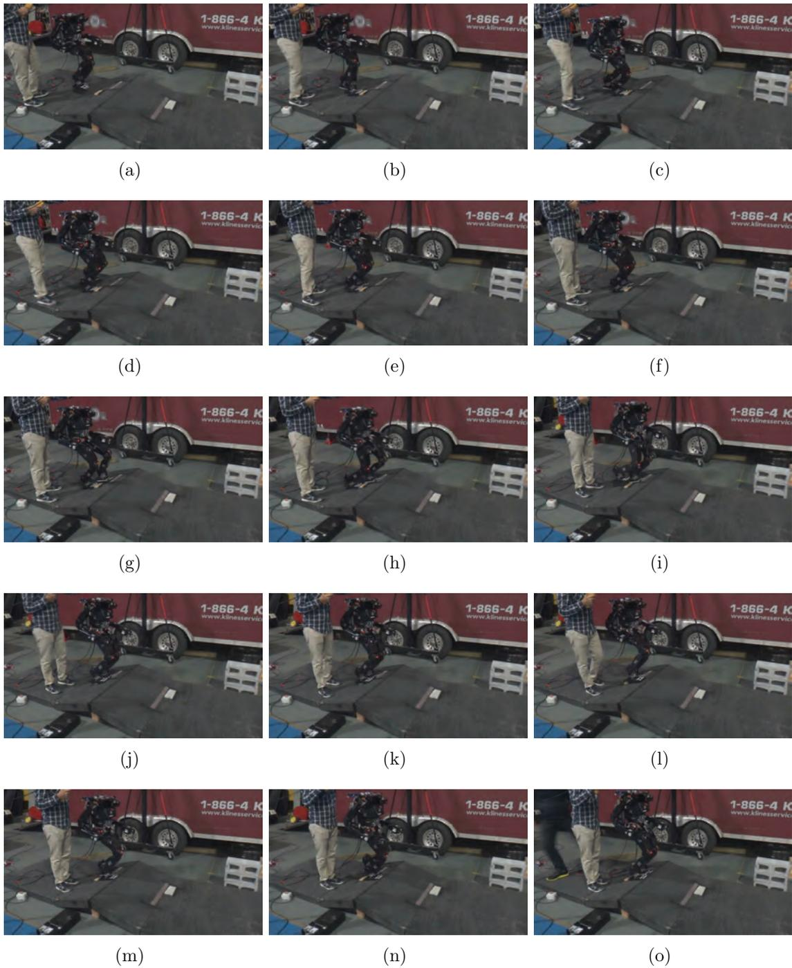
Figure 5.19: DRC-Hubo walking on 15deg inclined ramp with an arbitrarily rough surface.
