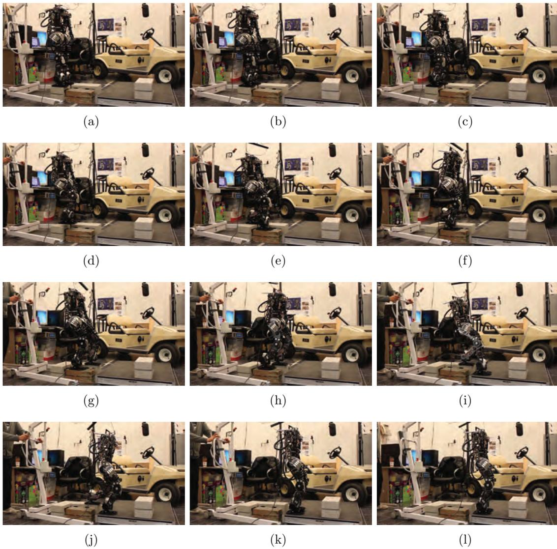
Figure 4.23: Online-Hubo walking on uneven terrains.
