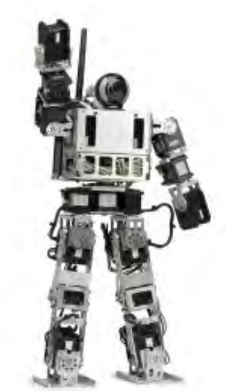
Figure A.2: Custom designed miniature humanoid robot for testing-and-evaluating, Mini-Hubo
