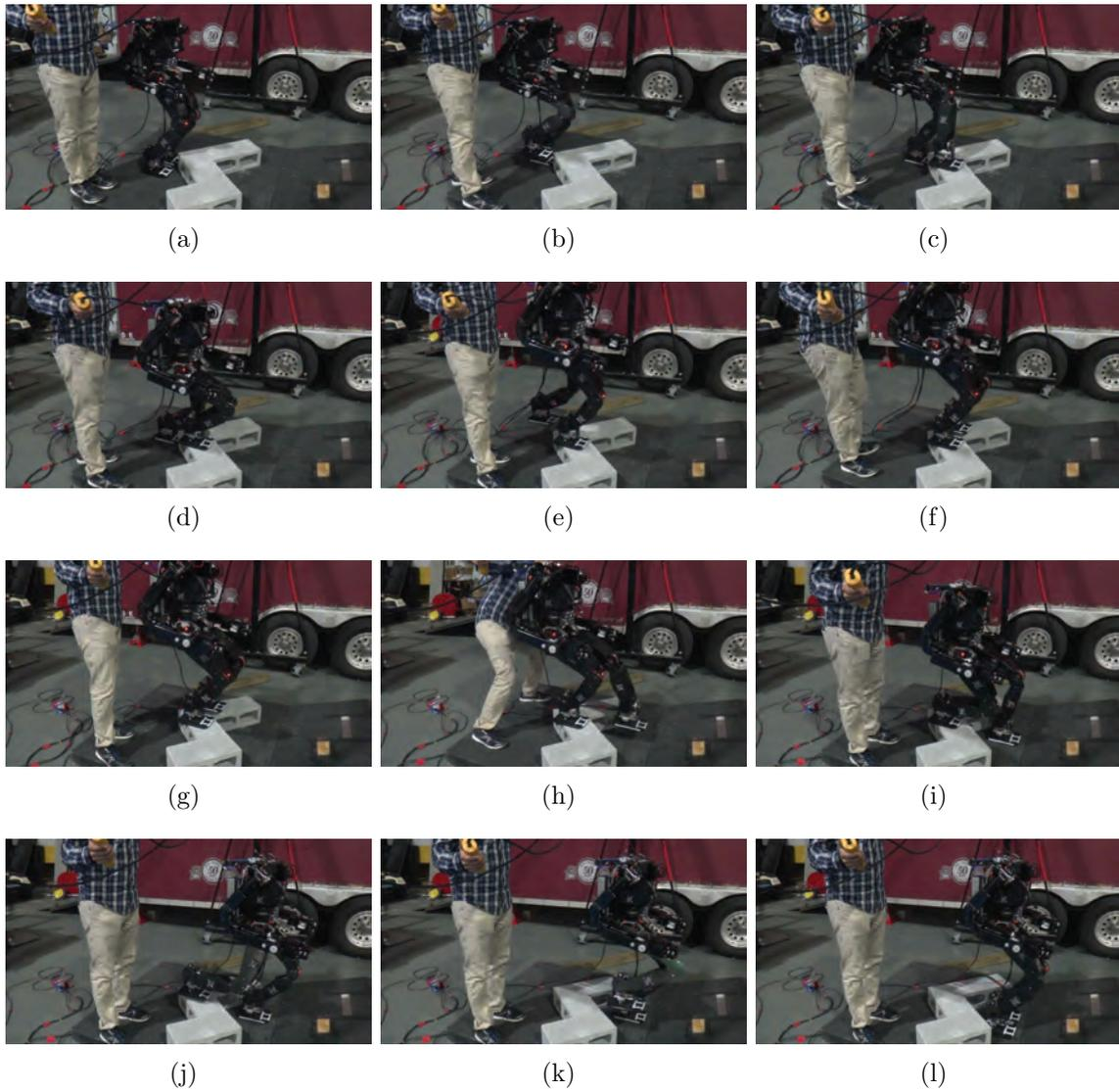
Figure 5.17: DRC-Hubo walking through an obstacle - a cinder block, 6 in. tall and 10 in. wide.
