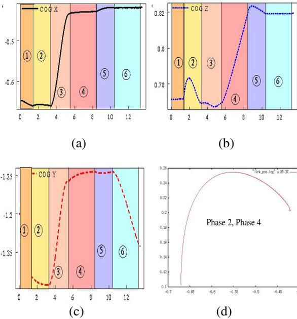
Fig.4 The prepared trajectory of step ascending Task for humanoid robot
