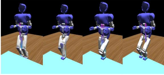
(b) The Task of step ascending for humanoid robot
