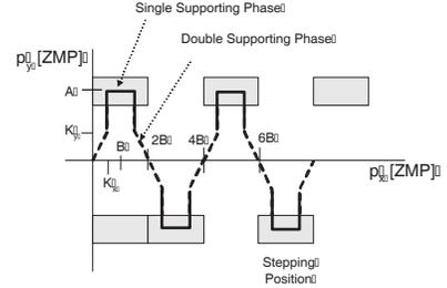
Fig. 2. Desired ZMP Trajectory
