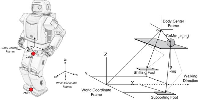
Fig. 1. Rolling Sphere Model for Dynamic Walking
