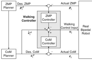
Fig. 4. Walking Controller for a Bipedal Walking Robot
