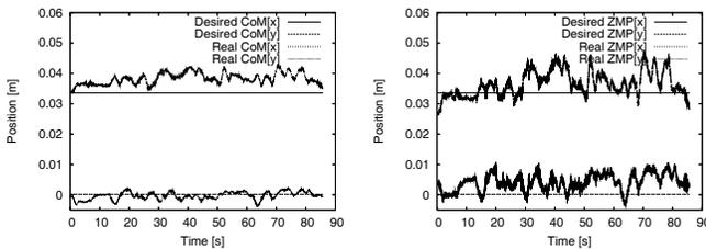
Fig. 6. Experimental Result : CoM and ZMP Trajectories while Dancing
