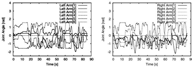
Fig. 5. Experimental Result : Joint Trajectories of Arms while Dancing
