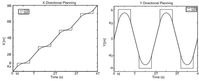
Fig. 3. X- and Y-Directional Desired ZMP/CoM Trajectories
