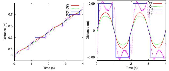
Fig. 7. Experimental Result : CoM and ZMP Trajectories while walking, where  $c_i$  means the actual position of CoM,  $c_i^d$  the desired position of CoM,  $p_i$  the actual ZMP, and  $p_i^d$  the desired ZMP for  $i = x, y$ .
