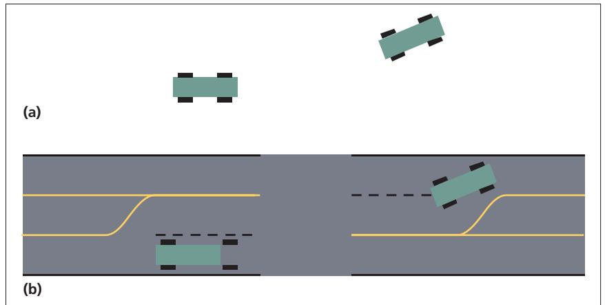
**Figure 2.** The importance of context for urban driving: (a) Without any context, the two vehicles appear to be on a collision course. (b) Given the context, we can safely assume that one of the vehicles is just making a lane change.
