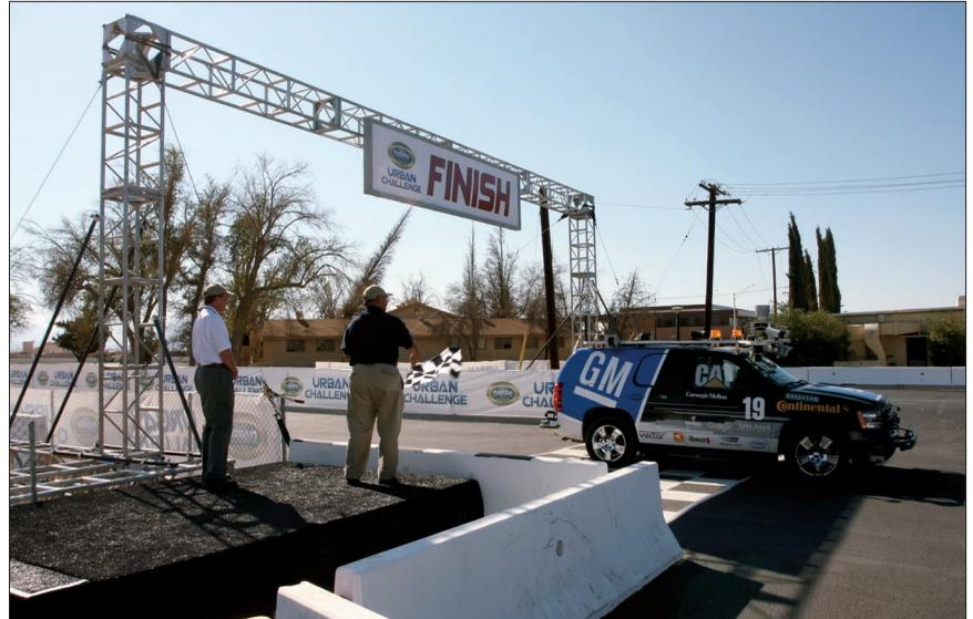
**Figure 1.** Boss, a modified Chevy Tahoe. Boss completed the 2007 DARPA Urban Challenge, safely navigating 53 miles through an urban environment among other moving vehicles.
