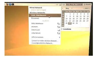
Now that the operating system of DARwIn-OP is connected to the wifi, open the terminal on DARWIN-OP, then type in "ifconfig" to the command line and scroll down to "wlan0" section to find the "inet addr" as shown.
