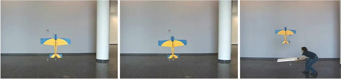
Fig. 15. First two images in the above sequence show the hybrid MAV in a fully autonomous hover at a height of 36 in at 6 s apart. In the third image, a board was placed under the MAV's tail that caused the controller to adjust the MAV's height to 36 in above the board. This was used to show that a constant throttle setting was not used to perform altitude hold.
