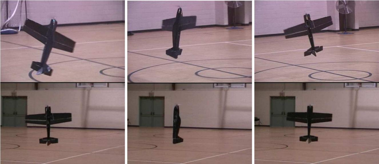
Fig. 8. (Top) Skilled human pilot hovers a fixed-wing aircraft in a small gymnasium and struggles to maintain a vertical orientation. (Bottom) Under autonomous control, the same aircraft is able to sustain a hover while remaining fixed in the vertical position.
