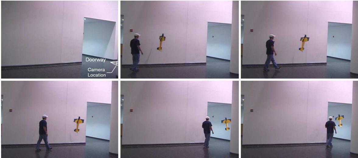
Fig. 18. Hybrid MAV autonomously follows the exterior wall of the building until detecting an open passageway. It then traverses the doorway to gather reconnaissance inside the building.
