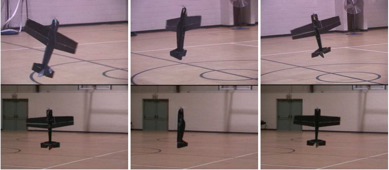
Figure 2: This figure shows video stills from blackhawk hovering under manual control (top) and autonomous control (bottom). The benefit of autonomous control can clearly be seen.
