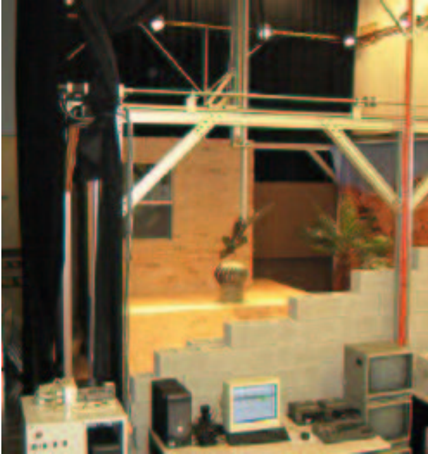
Figure 5: Systems Integrated Sensor Test Rig (SISTR). Sensor suites attached to the end effector feed data to the controller, which actuates the end effector based on the math model of the craft. This allows control algorithms to be tested against real world sensor data.
