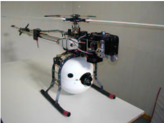
Figure 10: The SR100 electric helicopter from Rotomotion. The SR100 is sold off the shelf as a robotic platform capable of autonomous hovering and GPS waypoint navigation.
