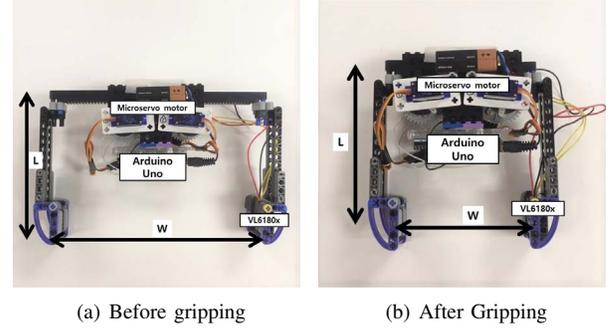
Fig. 5. LEGO-Based parallel gripper concept design
