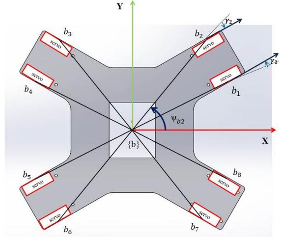
(b) Geometrical arrangement of leg attachment points
