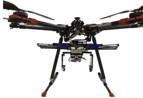
Fig. 2. Mobile manipulator for HTS proof-of-concept design
