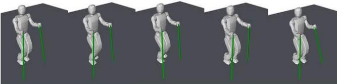
Fig. 10 Hubo ski-type walking on flat surface in OpenRAVE.
