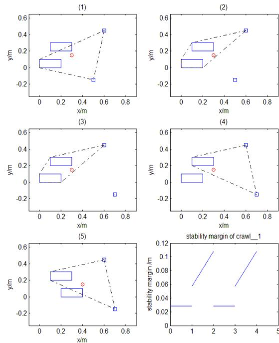
Fig. 5 Step sequence and stability margin of Crawl\_1
