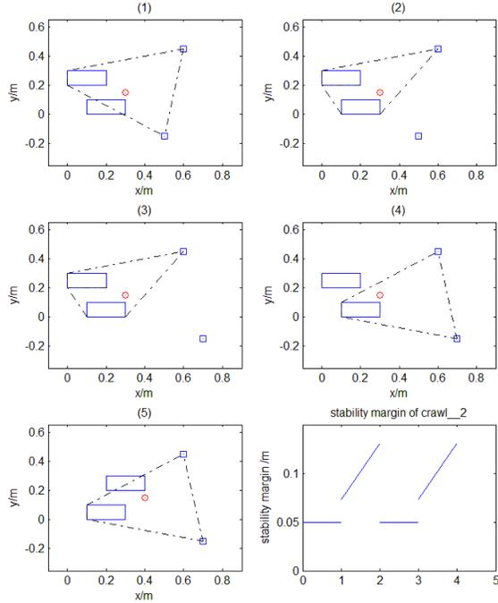
Fig. 6 Step sequence and stability margin of Crawl\_2
