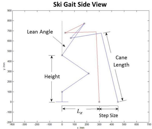
Fig. 8 Variables for developing ski-type gait
