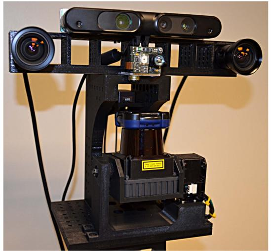
Fig. 2. Prototype sensor head with Asus Xtion Pro Live and tilting Hokuyo UTM-30LX-EW. Stereo color cameras, a PMD CamBoard nano, and a Microstrain IMU are also included but not used here.
