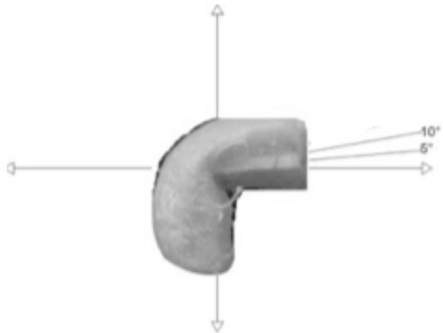
**Figure 9: Prototype bending 80 degrees**
