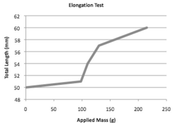
**Figure 8: Elongation test on silicone shell**
