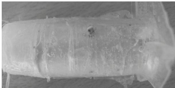
**Figure 7: Prototype composed of anisotropic shell and internally located aluminum joint and gel tube**
