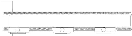
**Figure 5: Finger design with anisotropic silicone shell, embedded nylon fibers, gel tube, and three electromagnetic clutch controlled joints**
