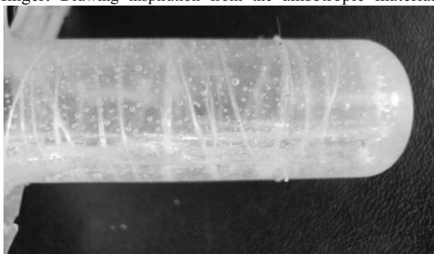
**Figure 6: Anisotropic silicone shell with embedded nylon fibers**
