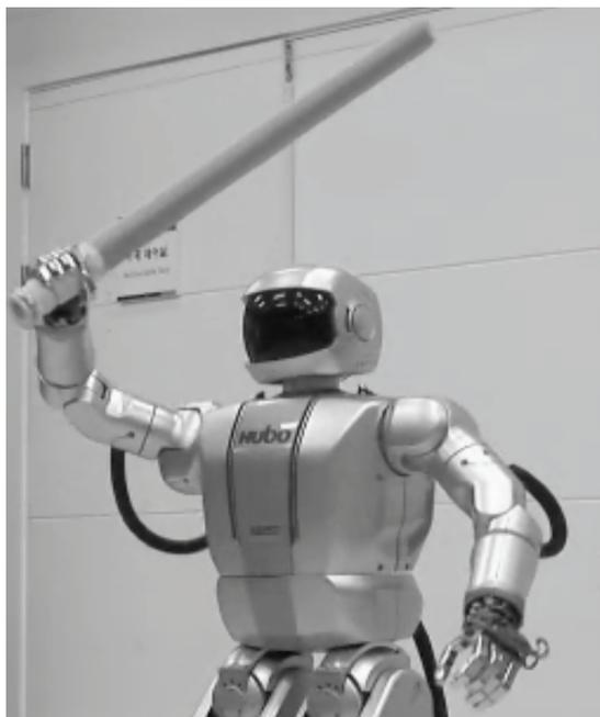
**Figure 1: Hubo is currently limited to shape adaptive grasp**
