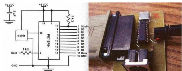
Figure 5: PC-to-RC schematic juxtaposed with actual circuit.
