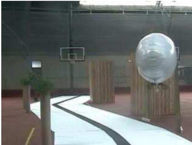
Figure 9: Swarthmore College’s blimp following the collision-free path.
