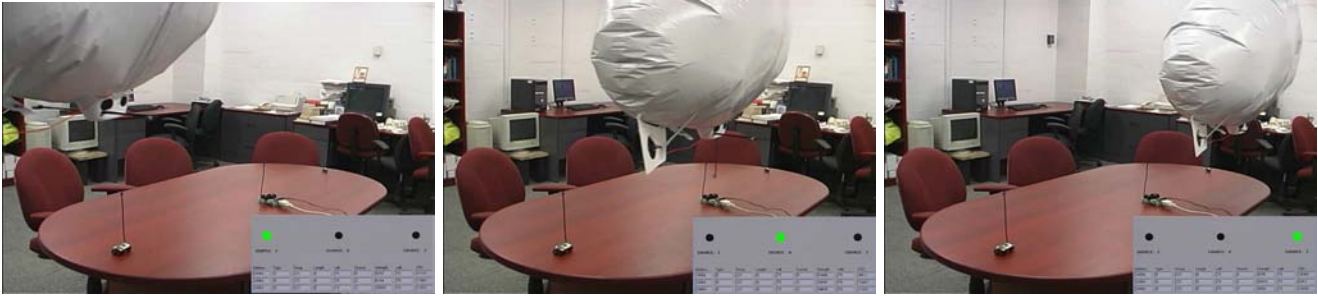
Figure 7: Signal strength is measured between a mobile node attached to the blimp and fixed nodes placed on a table. As the blimp passes by, the graphic corresponding to the nearest node is lit.
