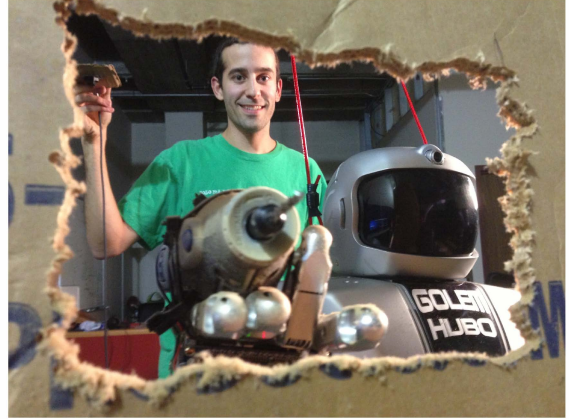
Fig. 1. Picture of Hubo and operator just after using telemanipulation to cut a rectangular hole out of a cardboard wall.
