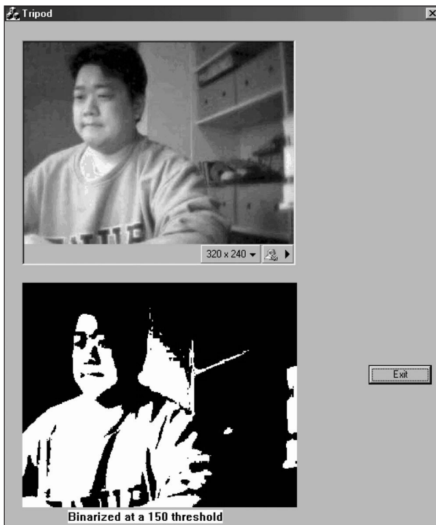
Figure 1. TRIPOD's Windows interface. Top and bottom viewports display the live camera field-of-view and processing results, respectively.
