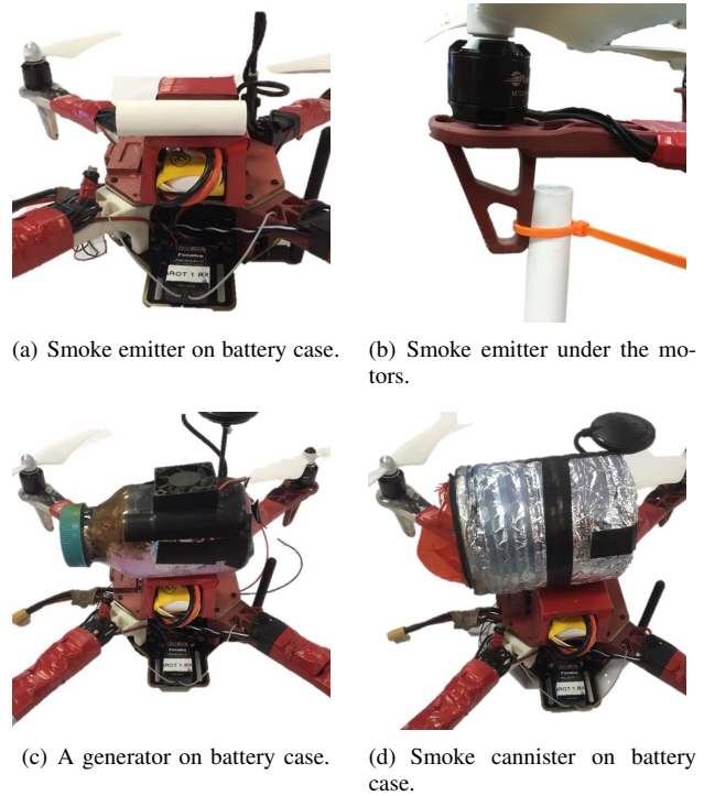
Fig. 4. Hardware designs for Skywriting
