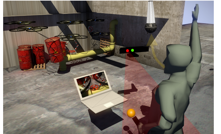
Fig. 5. Human in the loop control of unmanned aerial system using motion detection, voice control, and classical joystick inputs.
