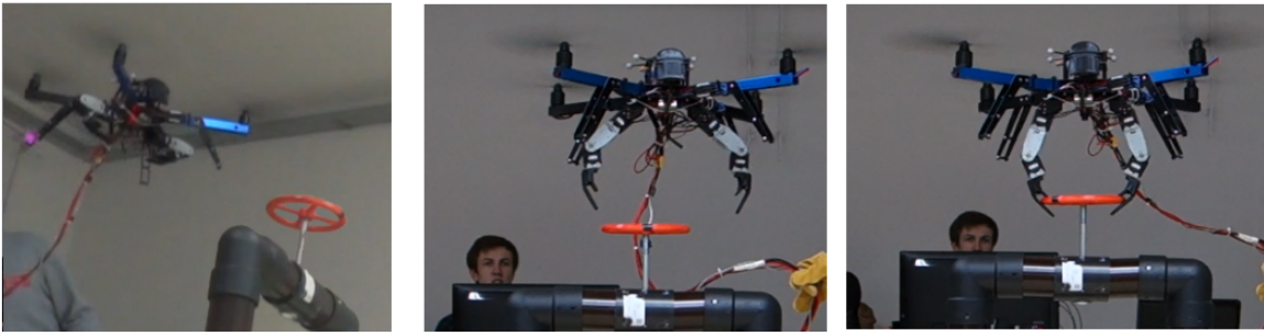
Fig. 6. MMUAV approaching and grabbing a valve: Taking off with arms stowed away for safety; approaching the valve; grabbing the valve.
