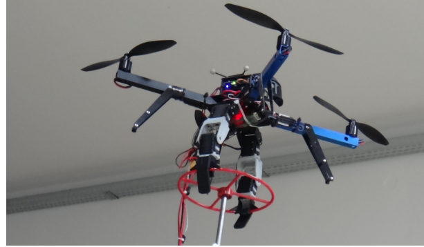
Fig. 1. MM-UAV dual-armed system performing a valve turning task.
