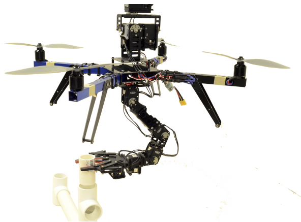
Fig. 1. MM-UAV in hover affixed to a 6-DOF overhead gantry
