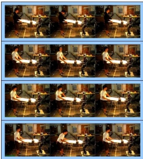
Fig. 5. Examples of Initially Designed Sign Languages for a Message indicating Start Carrying-Task: 1) Nodding Forward, 2) Nodding Backward, 3) Bending Arms, 4) Swaying Waist
