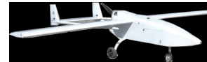
Fig. 6. The MAKO UAV developed by NAVMAR was modeled in X-Plane and used for experiment flights.
