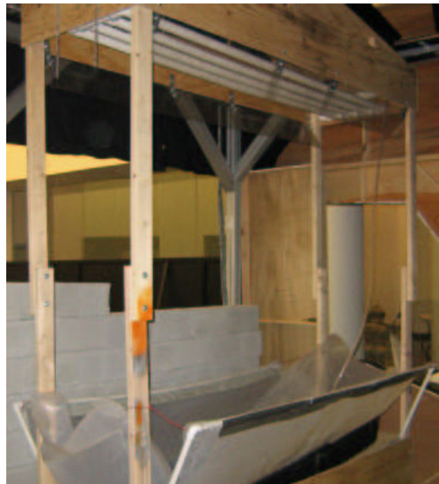
Fig. 2. Rain machine utilized for sensor testing. The machine can generate an 8ft wide by 2ft deep by 10ft tall sheet of rain with flow rates up to .2 in/min.
