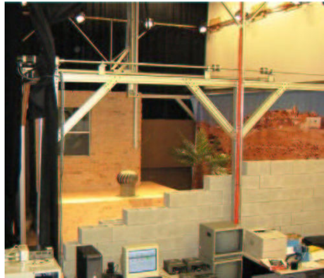
Fig. 1. Systems Integrated Sensor Test Rig (SISTR). SISTR permits real hardware to be tested in simulated urban environments and disaster scenarios. Environmental effects such as varied lighting, rain, and fog can be introduced in a controlled and repeatable fashion.
