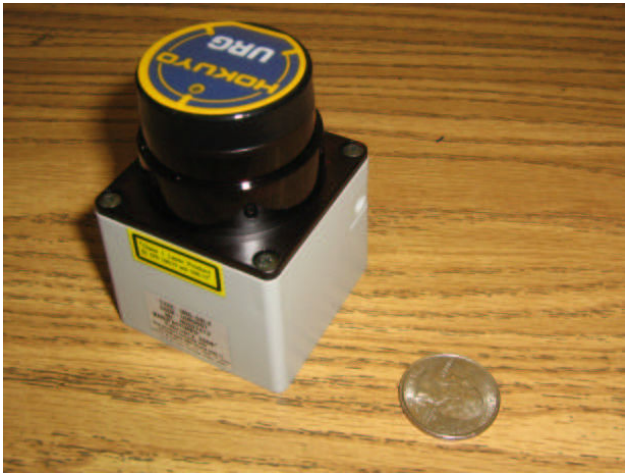
Fig. 3. The Hokuyo URG-04LX used for testing. Its small size (50mm x 50mm x 70mm) and light weight (160g) make it an attractive sensor for aerial platforms.
