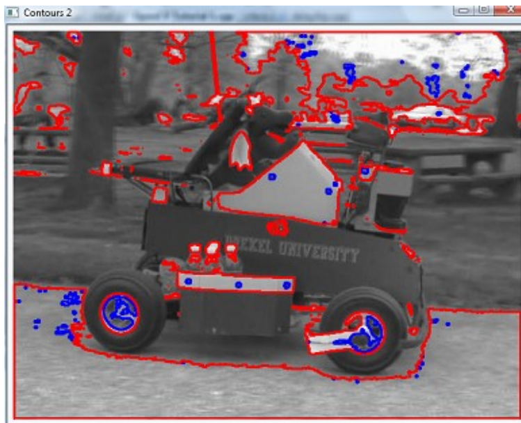
Finding and Drawing Contours on an Input Image
