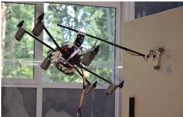
Figure 1. A photo demonstrating the multimodal locomotion system performing a cleaning operation on a vertical surface.
