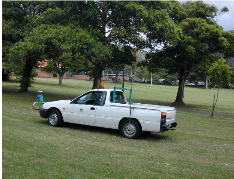
Figure 4: Utility car used for the experiments. The vehicle is equipped with a Sick laser range and bearing sensor, linear variable differential transformer sensor for the steering and back wheel velocity encoders.
