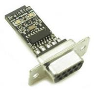
Figure 4 - Serial Level shifter
