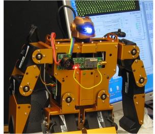
3. Place Bluetooth adapter (with complementary Velcro) firmly in place, and route the wire over the shoulder to the rear.
