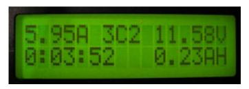
After the battery is charged, the charger will display a "CHRG Done" message. It will display the final pack voltage, total time elapsed until charge completes, and quantity of Amp-hours restored. This charger shuts off the fan and beeps, so you know to get the next battery going.
