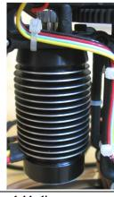
The brushless motor is mounted securely using the supplied screws and a few drops of Loctite<sup>TM</sup>or Threadlock<sup>TM</sup>.
