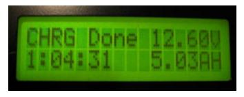
Cycle 1: 3 minutes blind charge at the specified charge rate
