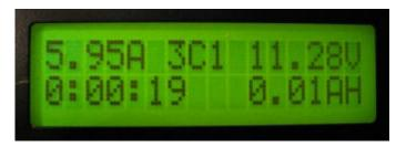
During the charge cycle it will continuously display the current charge rate, pack voltage, time elapsed and how much charge it's restored into the battery to that point in time. Having a charger that displays this much information about the charge is very handy for diagnosing possible problems.
