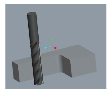
Most side milling on small machines is performed with an end mill. Cutting forces are higher due to the large area being cut. As such, depth of cut needs to be reduced, and should never exceed the radius of the cutter. Deep & heavy rough cuts will tend to bend the tool away from the work, which makes the cut shallower at the tip of the tool than at the base. Finish passes of about .005" to .010" depth of cut should be used to ensure a perpendicular edge.
