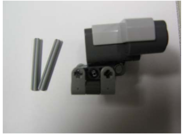
Figure 6J: From the side insert the two axles to suspend the sensor into place
