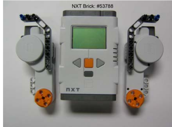
Figure 2D: Attach Motors to NXT Brick
