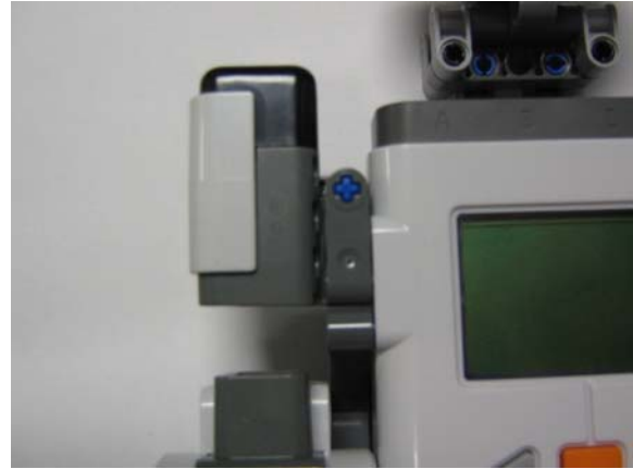
Figure 7D: Attach gyro to the left side of NXT Brick
