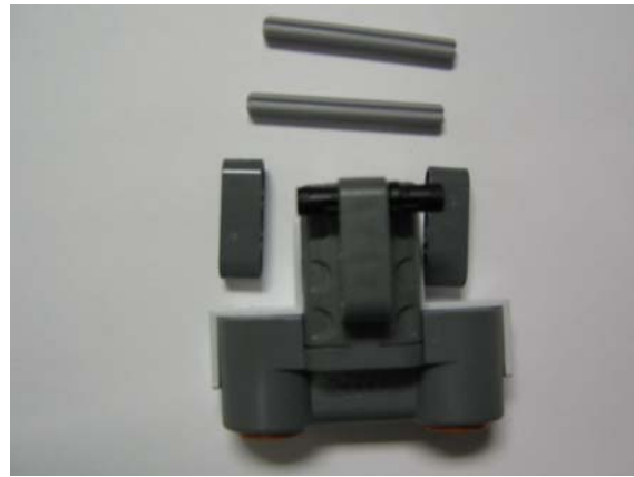
Figure 6D: Attach pin to end slot of sensor
