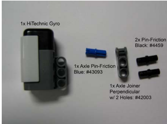
Figure 7A: Gyro mount components
