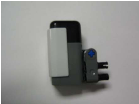
Figure 7C: Attach connector to gyro
