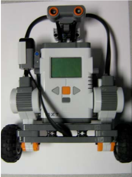
Figure 8B: Wire Gyro to Sensor Port 2
