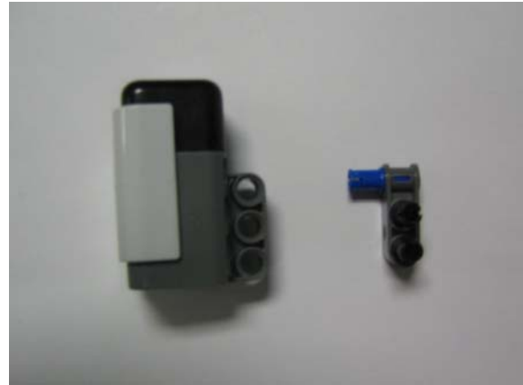
Figure 7B: Attach pins to connector
