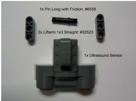
Figure 6C: Ultrasound Sensor components
