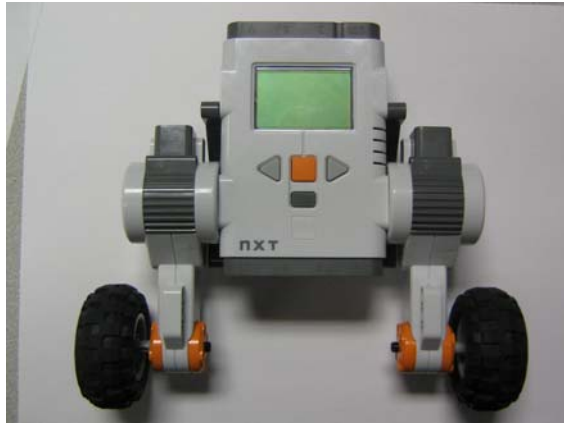
Figure 3E: Attach Wheel/Axle to Motors
