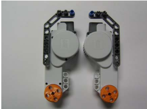
Figure 2C: Attach Arms to Motors
