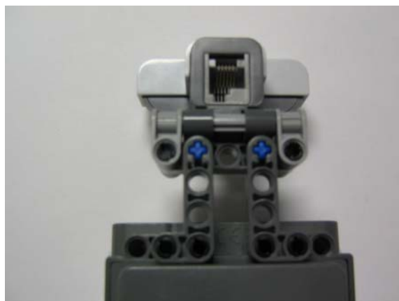
Figure 6M: Attach ultrasound mount to rear of NXT Brick
