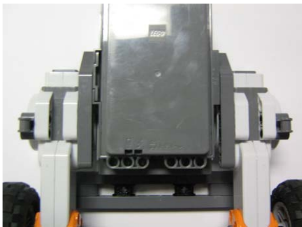
Figure 5H: Attach axle connector from 5F to rear of motors
