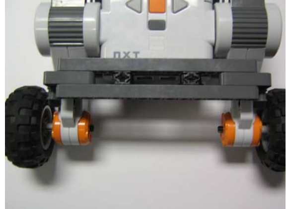
Figure 4J: Attach bracket to front of motor
