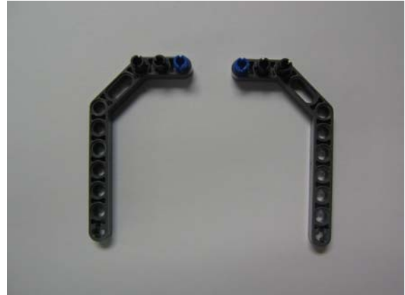
Figure 2B: Attach Pins to Arms
