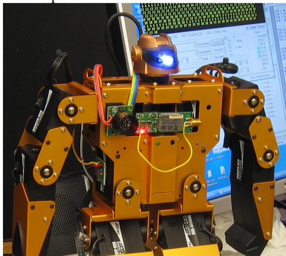
3. Place Bluetooth adapter (with complementary Velcro) firmly in place, and route the wire over the shoulder to the rear.
