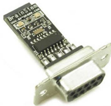
Figure 4 - Serial Level shifter
