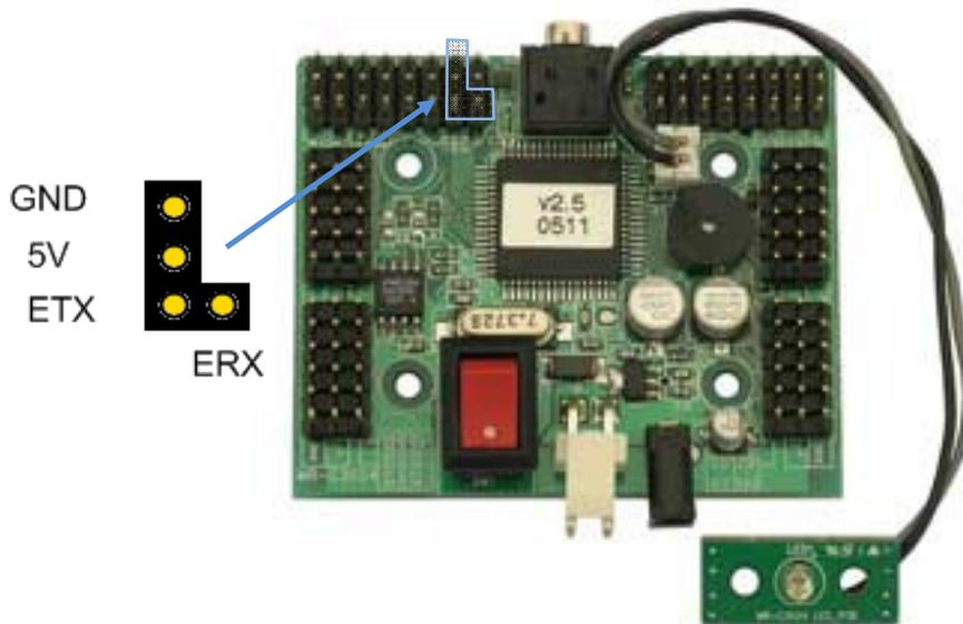
**Figure 5 - Controller Bluetooth connection at ETX/ERX pins**
