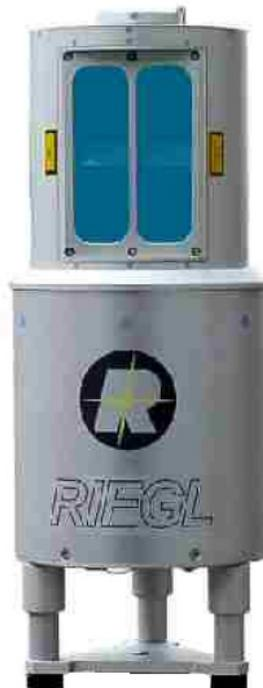
The Riegl LMS-Z210 is a high performance 3D laser measurement system. The LMS-Z210 is supported by Riegl's RiSCAN PRO software for performing scans over a 360° range in the horizontal plane and 80° range in the vertical range. Utilizing a class 1 laser, the sensor is able to resolve objects with 80% reflectivity up to 650m away! 3D laser scanners such as the LMS-Z210 are quickly replacing their 2D predecessors.
