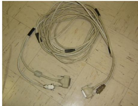
Connect the sensor to the computer using the serial and parallel cable. Plug the power cable into the bottom of the sensor. Connect the other end of the cable to the power supply. When the power supply is turned on, you should see the sensor head begin to rotate. The mirrors should then begin turning, and the sensor should continually scan. You're now ready to start working with the Riegl.
