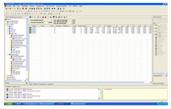
Now go to the second scan and select the same reflectors. You must give each reflector the same name on each scan or they will not be correlated correctly. One of the scans must now be selected to be the starting position, its coordinate system will be used as the world coordinate system; this is done by right clicking on it and selecting "Registered".
