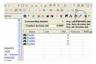
Move the check mark from "Project coordinate system" to the scan you just Registered and press start.
