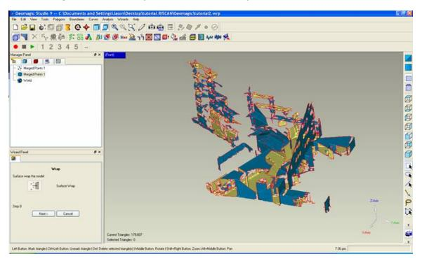
I will use the cut down version in later steps. Now it is time to do some touch up work on the model. There are a number of holes in the model that can be repaired. Go to "Polygons" and select "Fill Holes..."
