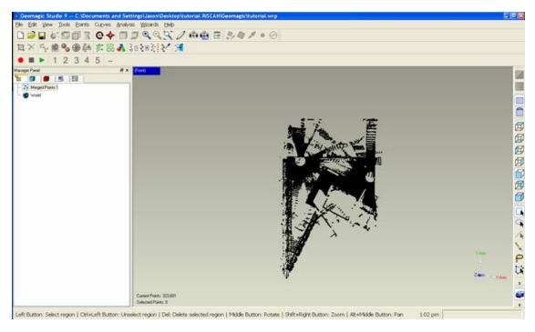
Now go into "Wizards" and select "Points to Polygons". Follow the wizard through the steps, just keep in mind that this software is designed for very high density point clouds, several million points on a 6 inch part, and we are working with  $\sim$ 300,000 pts over 10s of meters so use you judgment as to how to prune the point cloud. This is where you will need to decide what to do based on how you plan to use the result.
