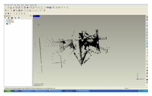
We can see here that the alignment looks good, as the shape are the space scanned is clear and the scanner locations, as indicated by the open circles, are correct. We also note that due to the large glass walls on the left and lower right sides of this image we have a significant reflection problem which we will confront later.
