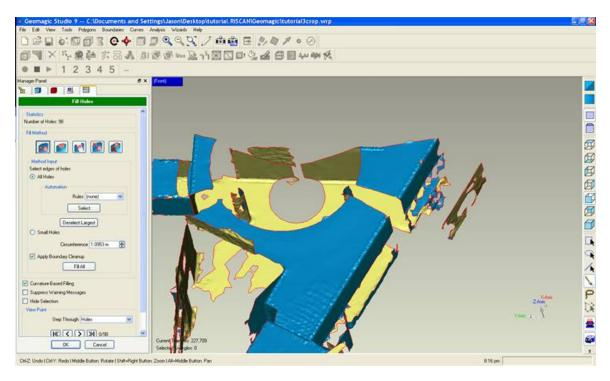
Select the Bridge command and select two points on a large or open sided hole to make a connection.
