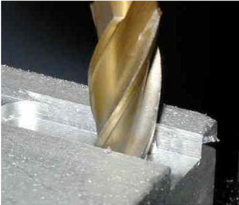
FIGURE 4 - SLOTTING ALUMINUM WITH AN END MILL
