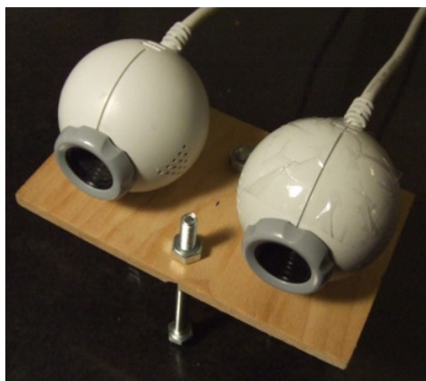
The camera setup I used for creating depth maps.
