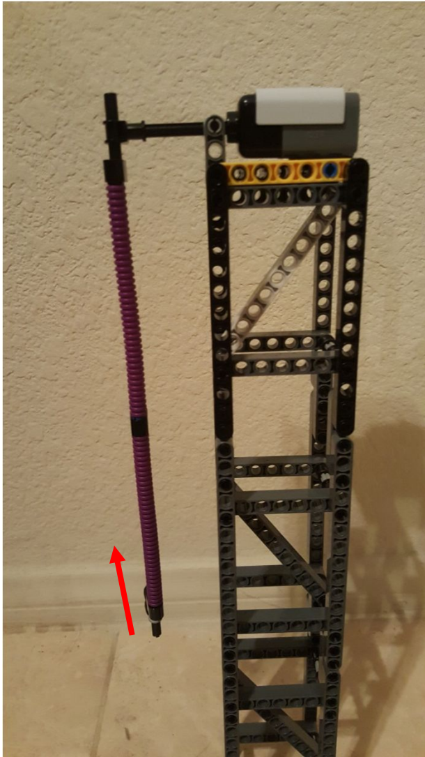
Perspective 1: When motorized propeller is mounted on Pendulum, Red Arrow shows that Pendulum will swing toward wall
