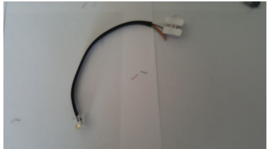
Alternative view: Only the Black and White wires in the NXT Cable will be used. Hence they are stripped
