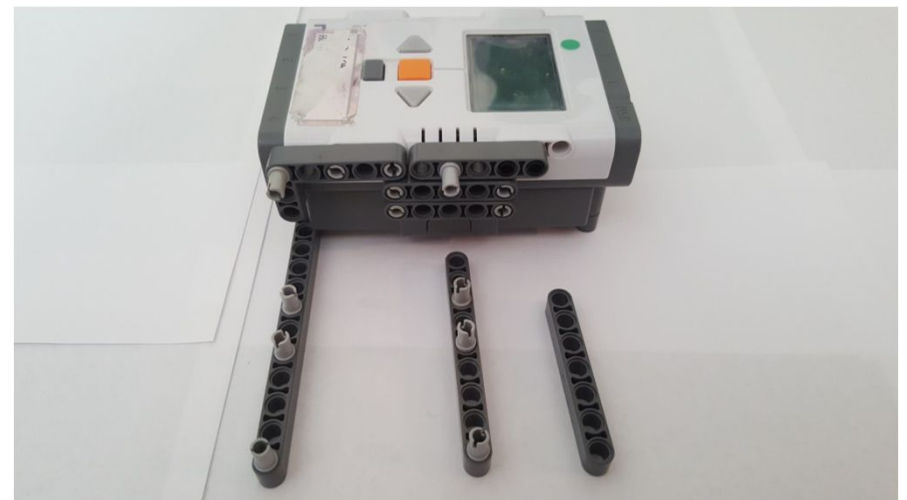
Insert the 8 Friction Pins as shown
