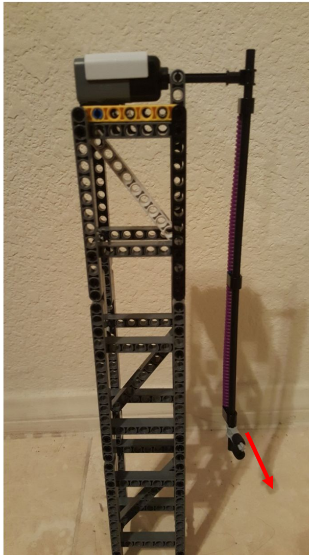
Perspective 2: When motorized propeller is mounted on Pendulum, Red Arrow shows that Pendulum will swing away from wall
