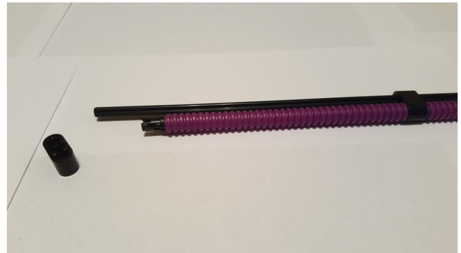
Repeat by inserting remaining Friction Pin into end of other Ribbed Hose
