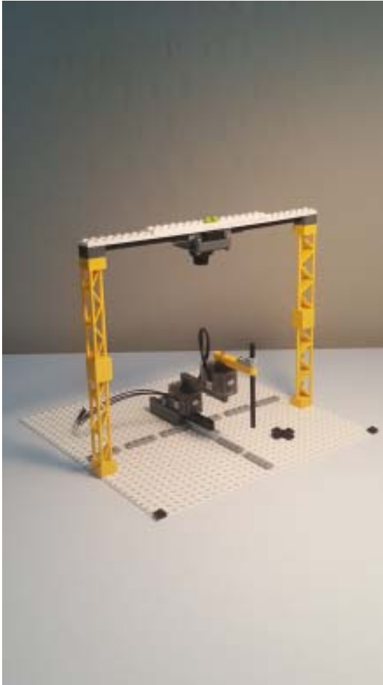
Completed Lego Camera Tower overlooking 2-DOF planar manipulator
