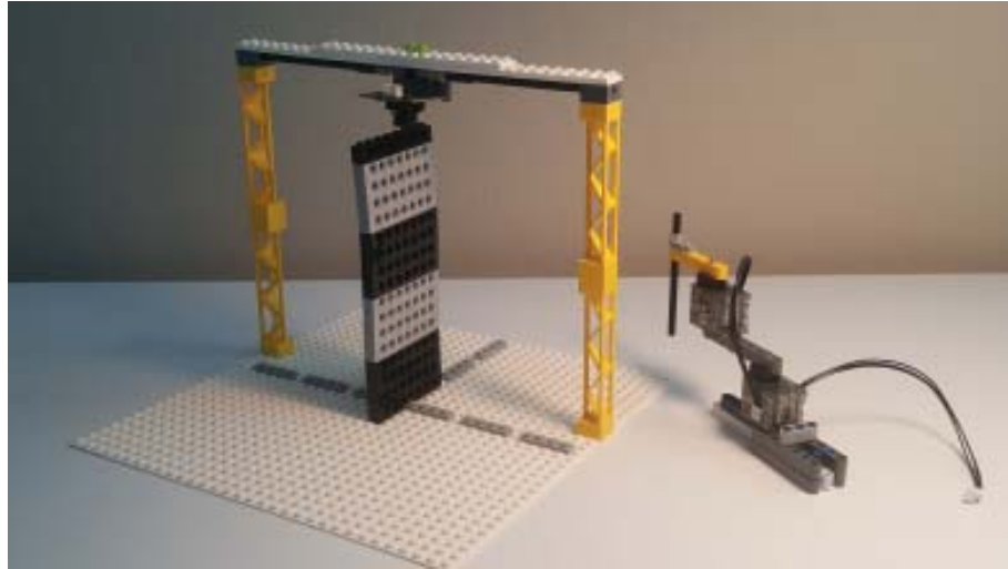
Stack of 17 Technic Bricks between Base Plate and Lens. 17 \times 6 \text{ mm} + 1 \text{ mm (due to stud)} = 103 \text{ mm} distance
