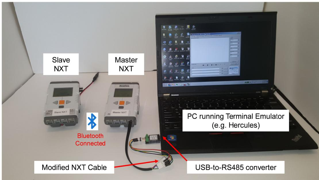
**Figure 2A:** Messages from PC are serially transmitted to the Master NXT. The Master NXT then wirelessly transmits them to the Slave NXT via Bluetooth. Video demonstration <https://youtu.be/P3qDNDvtpu4>
