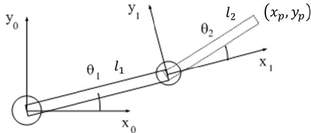
$$J_2^0 = \begin{bmatrix} J_v \\ J_\omega \end{bmatrix} = \begin{bmatrix} -l_1 s_1 - l_2 s_{12} & -l_2 s_{12} \\ l_1 c_1 + l_2 c_{12} & l_2 c_{12} \\ 0 & 0 \\ 0 & 0 \\ 1 & 1 \end{bmatrix}$$
