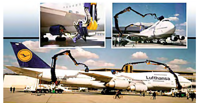
Fig. 4.11 The hydraulic Skywash aircraft cleaning robot
