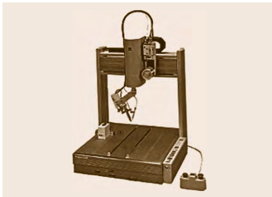
Fig. 4.19 The Sony robot uses open-loop permanent-magnet stepper motors
