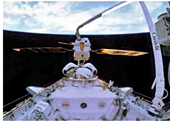
Fig. 4.27 The Space Shuttle robot arm has planetary gear joint drives
