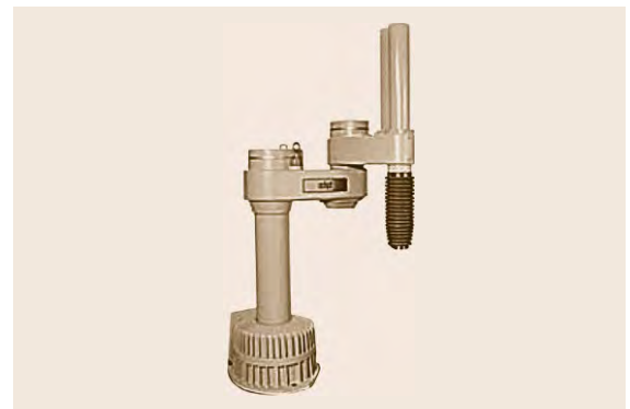
Fig. 4.20 The Adept robot uses closed-loop control and variable-reluctance motors (VIDEO 644)
