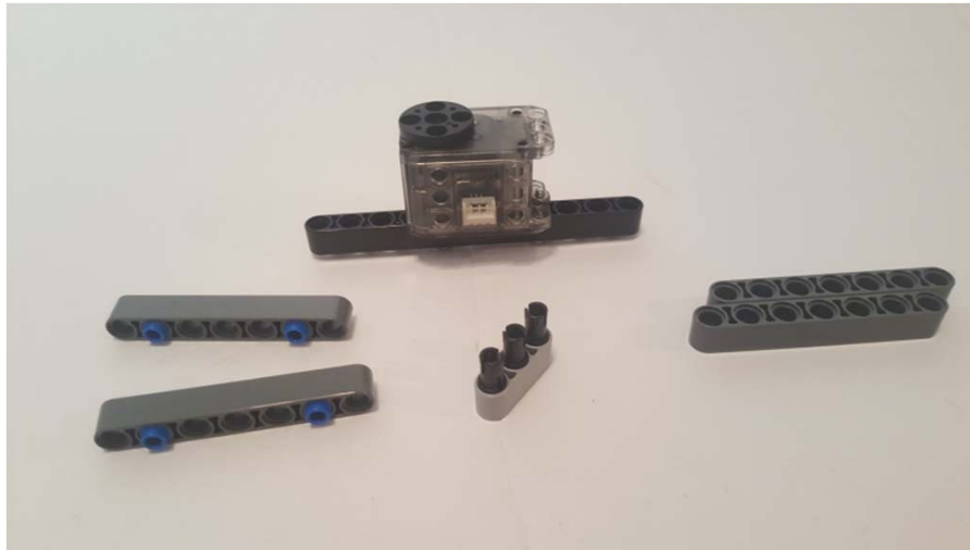
2A: Insert friction pegs in Beam 3. Insert Pin 1/2 in both Beam 7s.
