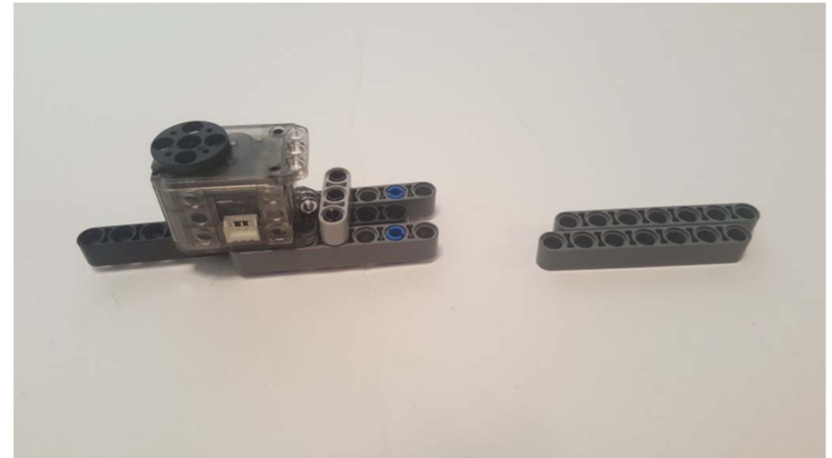
2B: Align two Beam 7s beneath motor and secure to Beam 3
