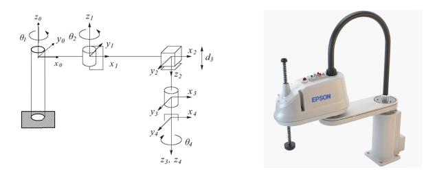
**Figure A:** Reference frames using Denavit-Hartenberg convention (left). Many manufacturing robot companies like Epson (right) offer SCARA products. Video of operation: https://www.youtube.com/watch?v=nSDM3eqcwuY
