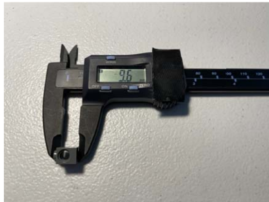
Figure 1C: From http://cs.wellesley.edu/~rds/handouts/LEGOSTructures.pdf , all Lego bricks are 6/5 FLU (or studs) tall (left). Since a FLU is 8 mm, this means the Brick is 9.6 mm tall (right). Note: height does not include the stud part.
