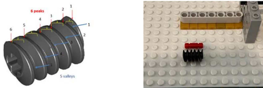
Figure 1B: Worm gear has 5 peak-to-peak spacings (yellow braces) and spans 2 studs
