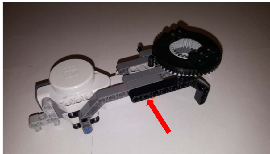
3F: Secure Double Angle Beam to Link 1 with Friction Peg
