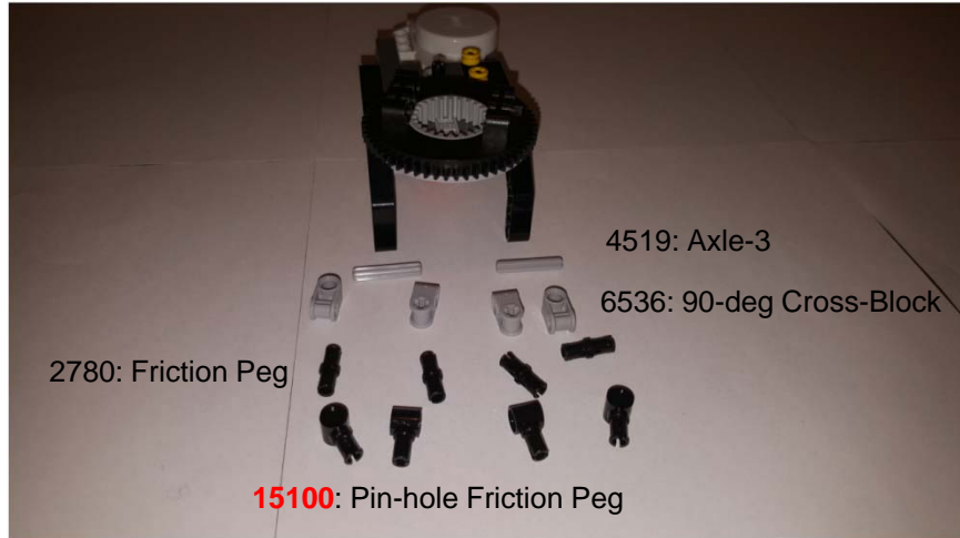
5A: Feet serve to secure Motor Base Assembly to a plate. NB: Need non-NXT part 15100
