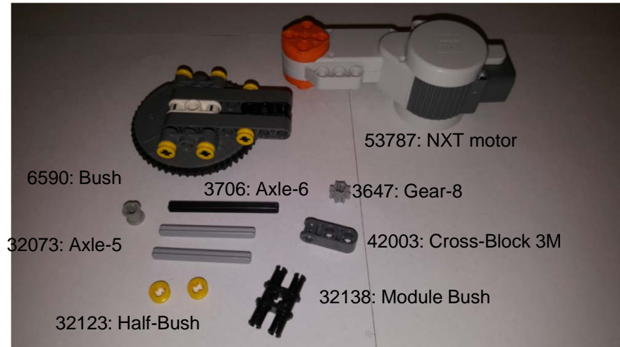
7A: Gather listed parts and Motor 2 with Joint 2 assembly from previous step
