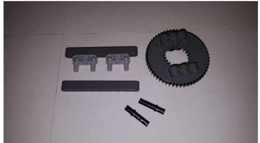
2B: Create Link 1 - mount 4-Snap Beams into a Beam-9.
