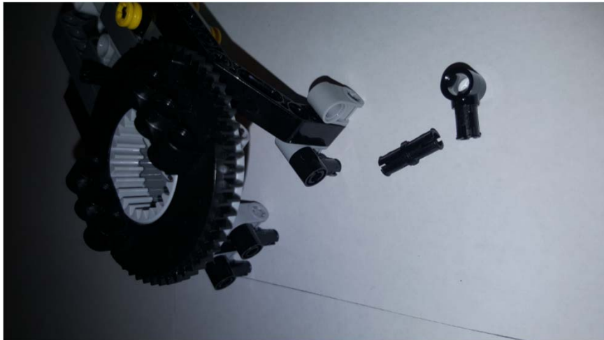
5C: Attach Pin-hole Friction Pegs to Motor Base Assembly's Double Angle Beam. Repeat Step 5B for remaining leg
