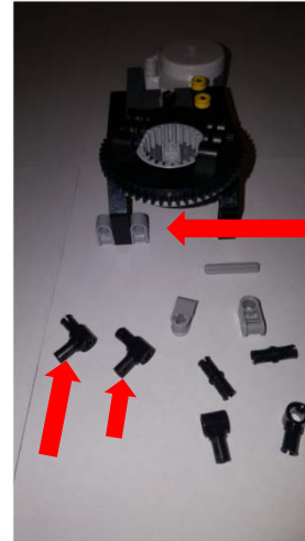
5B: Secure 90-deg Cross-Blocks to Motor Base Assembly with an Axle-3. Insert Friction Pegs into Pin-hole Friction Peg
