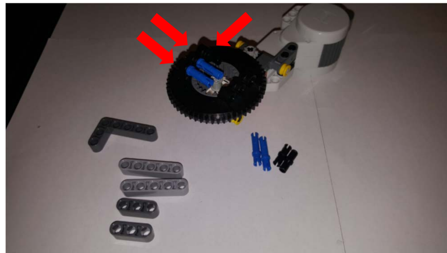
8B: Insert Long Friction Pegs and Friction peg in Turntable
