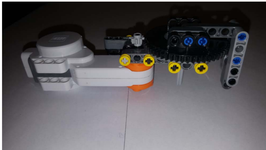
Alternative view of Link 2 assembly with end-effector
