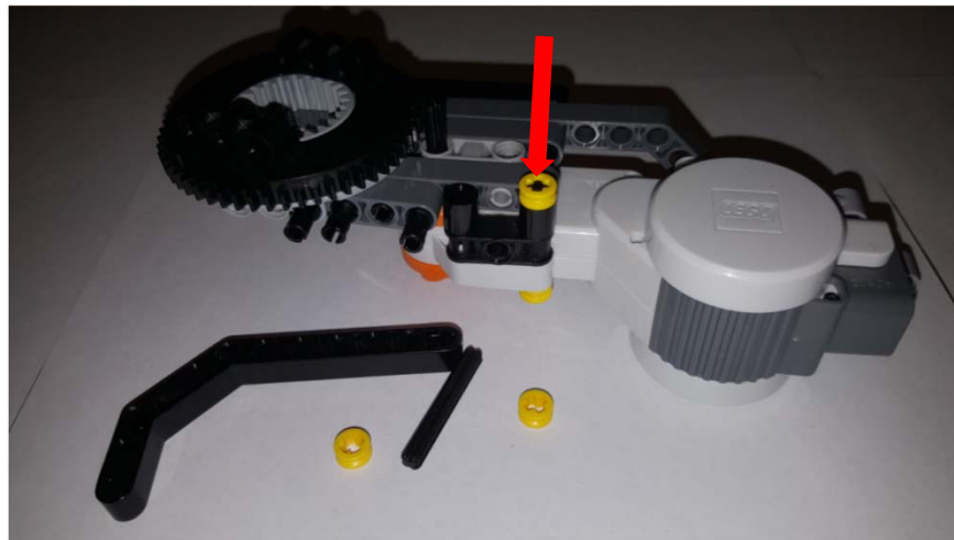
4A: Gather previous Base Motor assembly and Link 1 and listed parts. NB: Non NXT part 15100
