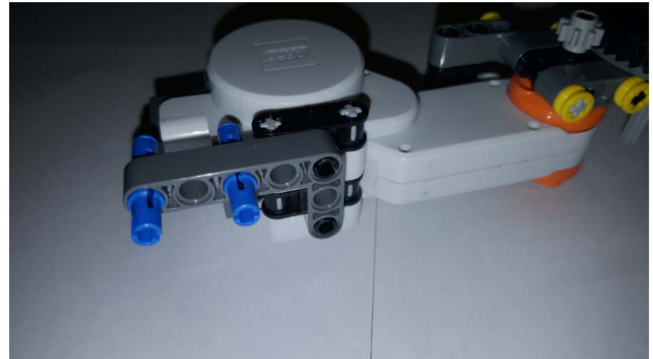
9D: Insert remaining friction peg to Double Cross-block and attach 3x5 Beam 90.
