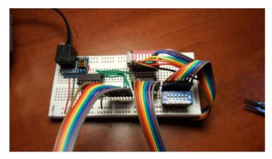
Step 1: Use Fig. 3A to connect two 8-wire ribbon cables to DIP switch and DIP LED
