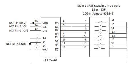
**Fig. 2A:** NXT-to-PCF8574 circuit diagram. Takes advantage of DIP switch package. PCF8574A's digital lines (D0-D7) are configured for input.
