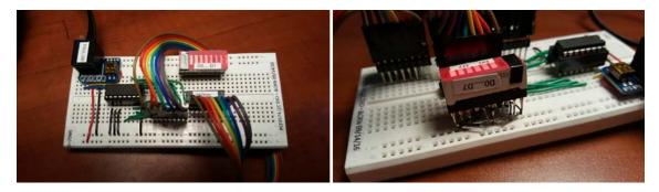
**Fig. 1B:** An 8-wire ribbon cable connects the PCF8574 chip to a 10-segment DIP display (left). Since only 8 LEDs are needed, black electrical tape covers two of them (right). To reduce wiring, one side of the 20-pin socket is used to connect the +5V bus. Some pins on this side are bend and wirewrapped to the other pins. Demo video: <u>https://youtu.be/AJlvYtODjlg</u>
