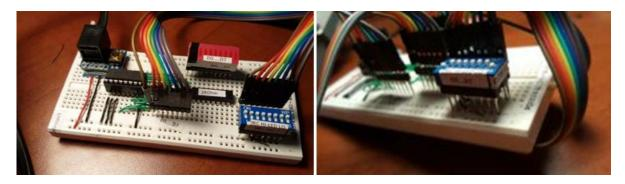
**Fig. 2B:** 8-wire ribbon cable connects 8-position DIP switch to PCF8574A's digital input lines (left). To reduce wiring, one side of the 16-pin socket is connected to GND (right). Demo Video: <u>https://youtu.be/rHXL8an3Kfs</u>
